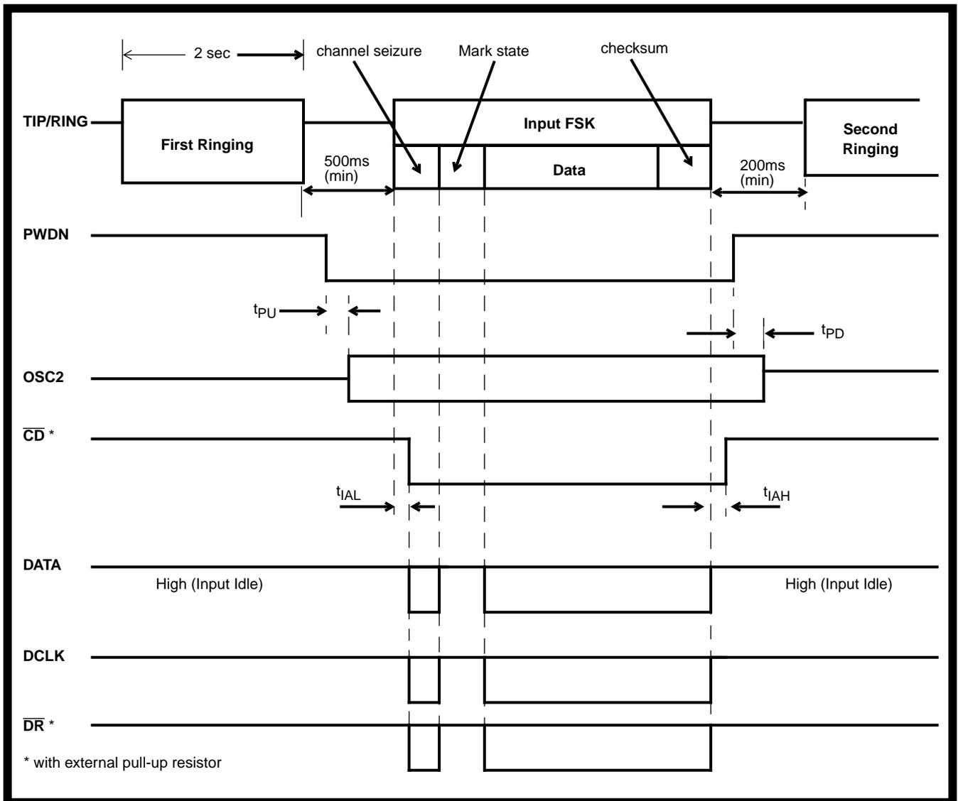
Figure 9 - Input and Output Timing (Bellcore CND Service)
