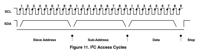
Following a start condition, each I<sup>2</sup>C device decodes the slave address. The TFP410 responds with an acknowledge by pulling the SDA line low during the ninth clock cycle if it decodes the address as its address. During subsequent sub-address and data cycles, the TFP410 responds with acknowledge as shown in Figure 12. The sub-address is auto-incremented after each data cycle.
