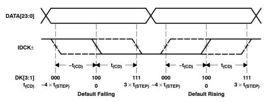
Figure 8. A Graphical Representation of the De-Skew Function
