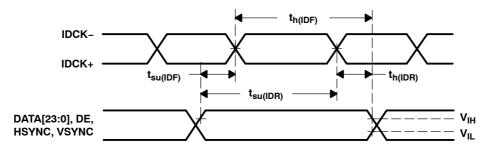
Figure 2. Control and Single-Edge-Data Setup/Hold Time to IDCK $\!\pm$
