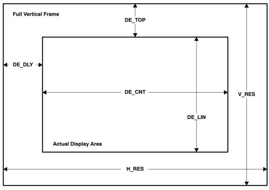
Figure 9. DE Generator Register Functions
