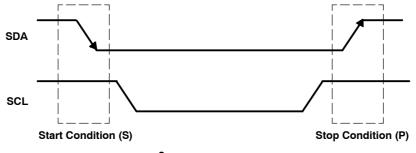
Figure 10. I<sup>2</sup>C Start and Stop Conditions
