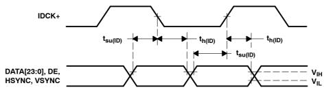
Figure 3. Dual Edge Data Setup/Hold Times to IDCK+
